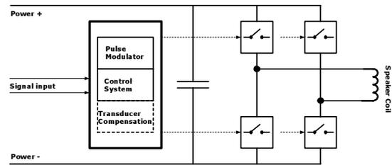
Figure 4 DC Active Transducer (DCAT) core electronic architecture
