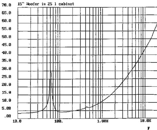
Figure 10 Impedance of 15" bass transducer.  $L_c = 1000\mu H$ .
