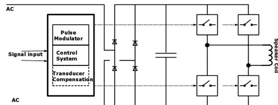
Figure 5 AC Active Transducer (ACAT) core electronic architecture
