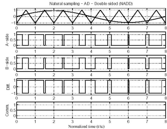
Figure 11 Time and frequency domain characteristics for Naturally sampled AD PWM (NADD) illustrated by HES surface [1]
