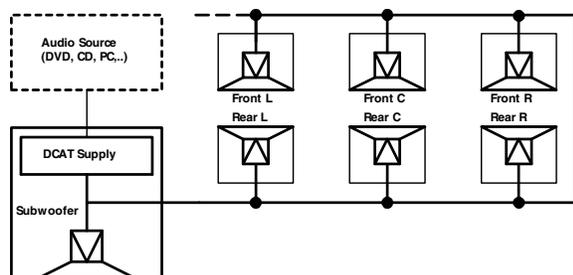
**Figure 25 Multi-channel architecture based on Active transducers**
