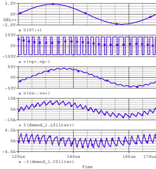
**Figure 8 Essential PMA output stage signals in a 250W/80V case example, from top to bottom (1) Input signal, (2) Power stage output (3) Demodulated output (4) Inductor current and (5) Filter capacitor current**
